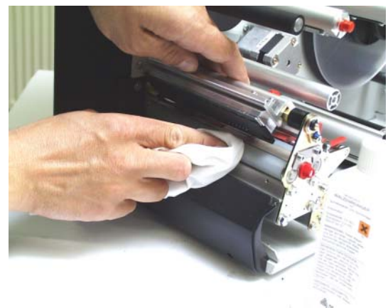
Fig. 4 Rotate the printhead upwards before cleaning it.
