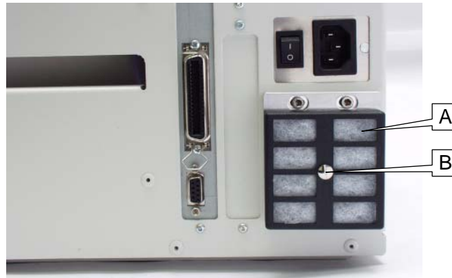
Fig. 7 64-08 with mounted dust filter (A).
