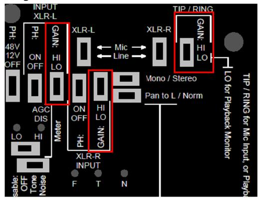
The Block Diagram illustrates where the low-noise preamplifiers are located in the system. Note that the two low-noise preamps for the <u>TIP-L</u> and <u>RING-R</u> inputs have their gain settings controlled by one switch (so both will either be <u>HI</u> or <u>LO</u>).
