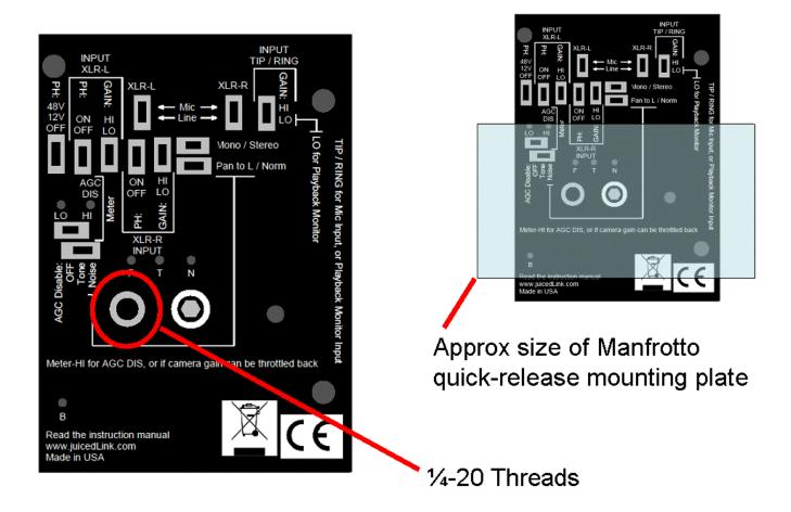
The bottom of the DT454 has ½-20 threads for mounting to the top of a tripod, or other device.
