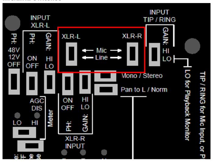
The <u>LINE</u> position inserts a 40dB attenuator before the preamps in the  $\underline{XLR-L}$  and  $\underline{XLR-R}$  signal chains.
