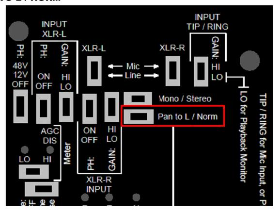
As illustrated by the Block Diagram, the <u>PAN TO L</u> switch position routes the right channel over to the left channel. So, <u>PAN TO L</u> is used to route <u>XLR-R</u> and <u>RING-R</u> to the left channel for recording.
