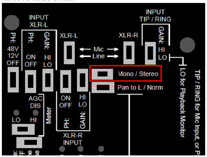
As illustrated by the Block Diagram, the <u>STERO</u> switch position keeps the right and left signal channels independent from each other, and presents them to the corresponding right and left output connections of the <u>OUT</u> minijack.
