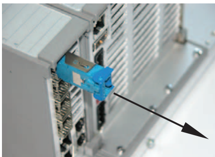
Figure 22: Disassembling an SFP module
