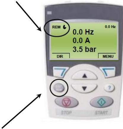
The **LOC/REM** button enables the user to switch between REMOTE (REM) and LOCAL (LOC) mode as required.
