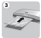
Place pouch, sealed edge first, into laminator entry. Keep pouch straight and use the edge guide to center it.
