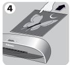
To prevent jamming, immediately remove laminated item from back of machine. Let item cool on flat surface for several seconds.
