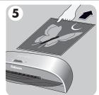
To prevent jamming, immediately remove laminated item from back of machine.
