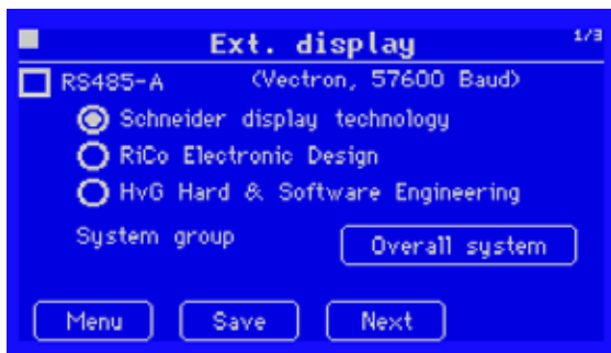
Figure 9-36: Ext. display at RS485-A
