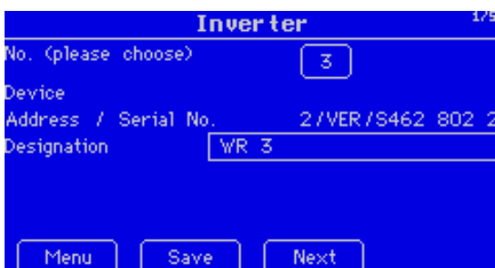
Figure 9-23: Selection of solar inverter
