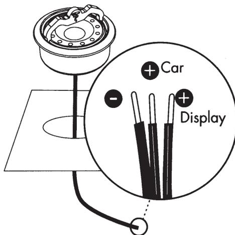
When installing on a demonstration display, connect the "display" wire.
