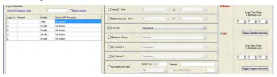
b) Logic true delay is 0s, in the 'trigger target when true' window, input dimmer/relay ID, here is 1-6, parameter 1 is channel 2, parameter 2 is 100.
