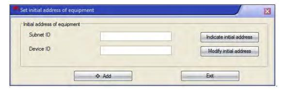
d) Click the "Indicate initial address", the device ID of the 12in1 sensor will then be shown. If you wish to modify the address, fill in the new address, and click the "Modify initial address". Click the "+Add" button, and the module will be included in the "ON-line devices" list.
