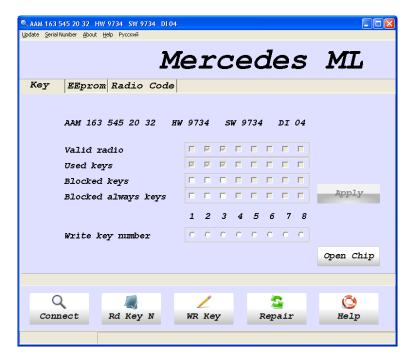
Here you additionally see Valid radio window, according to the information in the window you can make a conclusion that there are two keys (of all the three "active" keys) positioned 2 and 3 which have remote control programming of the central lock radiochannel.
