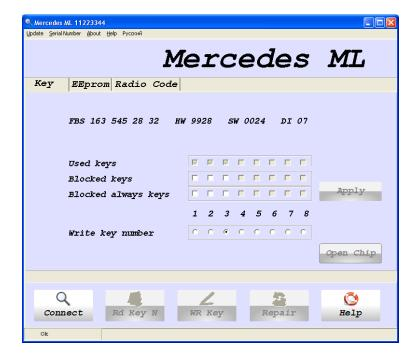
When the writing is finished we recommend some testing – press Connect then Rd Key N and make sure that the new key has number 3
