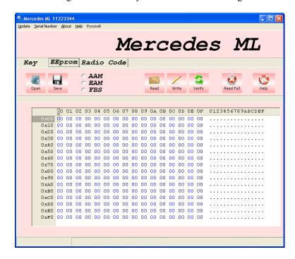
The interface is quite simple and hardly requires explanation. When the ECU you want to read is chosen you can read EEPROM field, as well as write and verify it. You can stop the reading process at any moment by pressing Esc button on your computer. After you press Read Full all the data from the processor is read which takes a lot of time!
