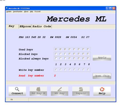
It means that the only original key is written by number 2. We make a decision to write an additional key by number 3 to replace the lost one! It is necessary to say that you can write a new key to any other position from 4 to 8 and block the key at position 3 by ticking the necessary boxes.
