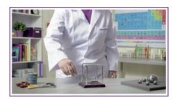
If more balls are lifted on one end, then the same amount of balls will be lifted on the other end of the series of the spheres.
