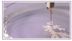
source (this will be the anode) in the liquid, while use a pin as the cathode, which need to be placed gently on the surface of the liquid so that surface tension keeps it there. After turning on the power source, silver is formed on the cathode, which keeps on "growing" on the surface of the liquid.
