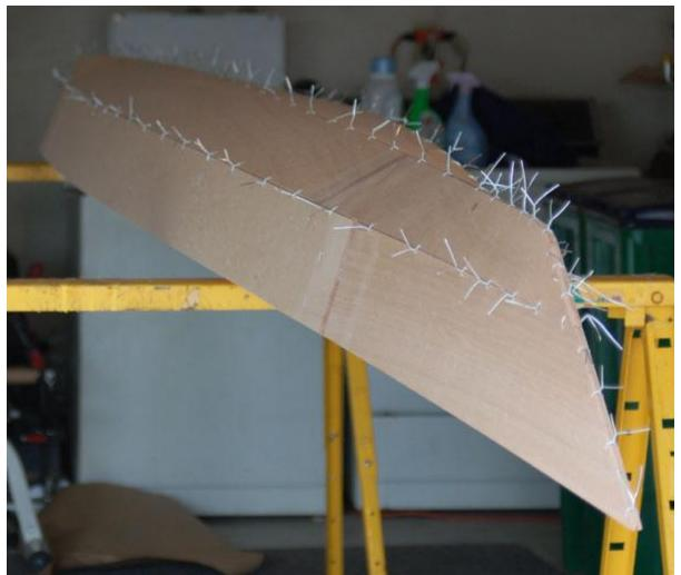
When the hulled is wired together is the best time to make sure the lines are straight and fair.
