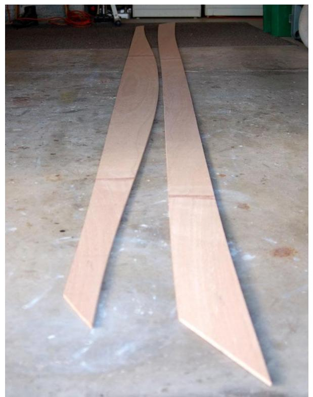
The bottom and side panels, stacked with the insides facing each other. The bow ends are in the foreground.
