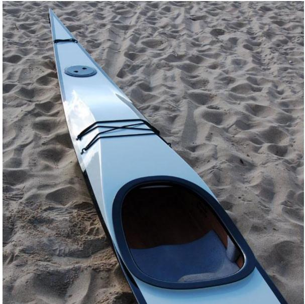
The "humpdeck" with room for the feet to be vertical and together for a better forward stroke.
