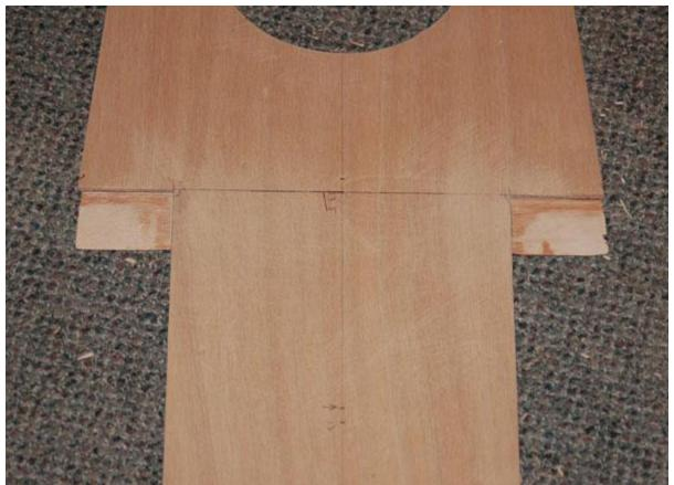
4 inch strip of plywood epoxied to the bottom of the deck at the 13 feet and 6 inches mark to help with attaching the deck side panels later.
