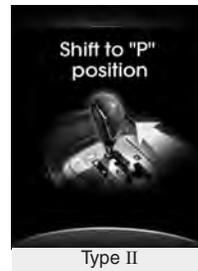
If you push the engine start/stop button with the engine start/stop button ON and the shift lever not in P(Park), the warning illuminates on the LCD screen for 10 seconds to indicate that you should press the engine start/stop button with the shift lever in P(Park) to turn off the engine.
