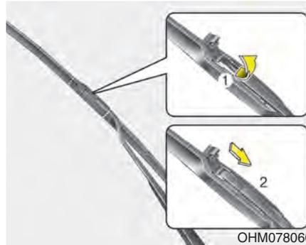
2. Open the cover of the blade. Press the clip behind the wiper arm and remove the blade assembly downward.
