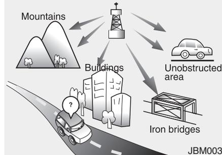
FM broadcasts are transmitted at high frequencies and do not bend to follow the earth's surface. Because of this, FM broadcasts generally begin to fade at short distances from the station. Also, FM signals are easily affected by buildings, mountains, or other obstructions. These can result in certain listening conditions which might lead you to believe a problem exists with your radio. The following conditions are normal and do not indicate radio trouble:
