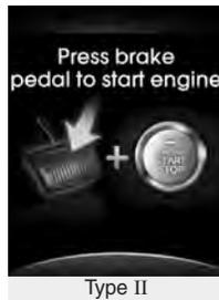
If the engine start/stop button turns to the ACC position twice by pushing the engine start/stop button repeatedly without pressing the brake pedal, the warning illuminates on the LCD screen for 10 seconds to indicate that you should press the brake pedal to start the engine.
