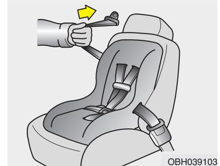
4. Slowly allow the shoulder portion of the seat belt to retract and listen for an audible "clicking" or "ratcheting" sound. This indicates that the retractor is in the "Automatic Locking" mode. If no distinct sound is heard, repeat steps 3 and 4.
