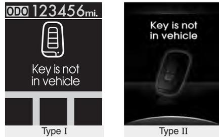
If the smart key is not in the vehicle and if any door is opened or closed with the engine start/stop button in ACC, ON, or START, the warning illuminates on the LCD screen. The chime also sounds for 5 seconds when the smart key is not in the vehicle and any door is closed.
