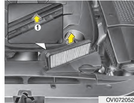
2. Replace the air cleaner filter after pulling up the locking tab (1).
