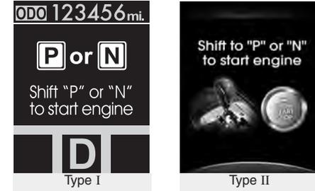
If you try to start the engine with the shift lever not in P(Park) or N(Neutral), the warning illuminates for 10 seconds on the LCD screen.
