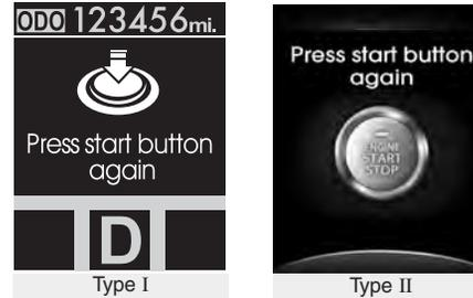
If there is a problem with the engine start/stop button system, the warning illuminates for 10 seconds to indicate that you could start the engine by pressing the engine start/stop button while pressing the brake pedal.
