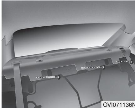
7. Loosen the mounting screws, then remove the package tray trim.
