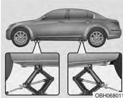
8. Place the jack at the front or rear jacking position closest to the tire you are changing. Place the jack at the designated locations under the frame. The jacking positions are plates welded to the frame with two tabs and a raised dot to index with the jack.
