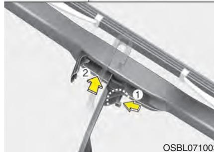
2. Turn the wiper blade clip. Then lift up the blade clip.
