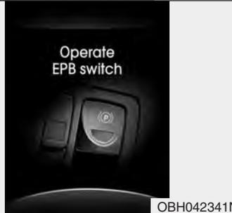
8. After using the EPB emergency release, a warning message will come on. You should operate the EPB switch for the vehicle to return to its normal condition. If the vehicle does not return to normal condition, take your vehicle to an authorized HYUNDAI dealer and have the system checked.
