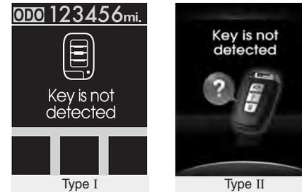
If the smart key is not in the vehicle or is not detected and you push the engine start/stop button, the warning illuminates on the LCD screen for 10 seconds.
