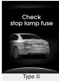
When the stop lamp fuse is disconnected, the warning illuminates for 10 seconds on the LCD screen.
