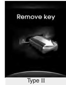
When you turn off the engine with the smart key in the smart key holder, the warning illuminates on the LCD screen for 10 seconds. Push the smart key inward and pull it out from the smart key holder.
