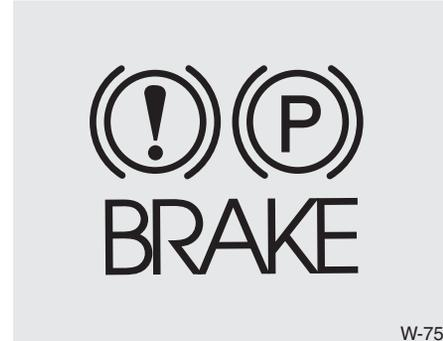
Check the brake warning light by turning the ignition switch ON (do not start the engine). This light will be illuminated when the parking brake is applied with the ignition switch in the START or ON position. Before driving, be sure the parking brake is fully released and the brake warning light is off.
