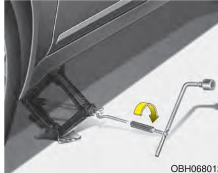
9. Insert the jack handle into the jack and turn it clockwise, raising the vehicle until the tire just clears the ground. This measurement is approximately 30 mm (1.2 in). Before removing the wheel lug nuts, make sure the vehicle is stable and that there is no chance for movement or slippage.
