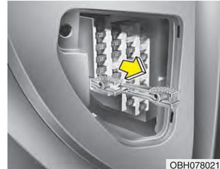
3. Pull the suspected fuse straight out. Use the removal tool provided in the front passenger's side panel.
