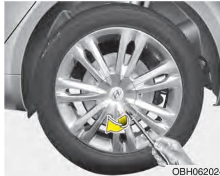
6. Insert the jack handle into the groove of the wheel cap and pry gently to remove the wheel cap (if equipped).
