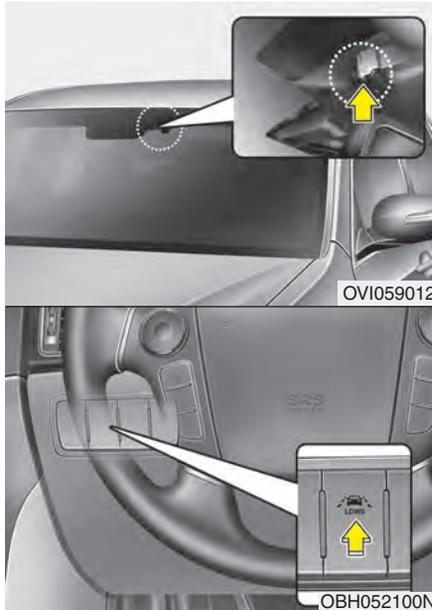
This system detects the lane with the sensor at the front windshield and warns you when your vehicle leaves the lane.
