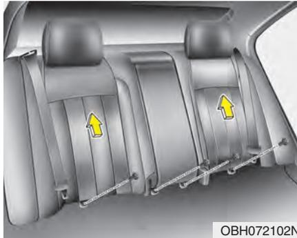
3. Loosen the mounting bolts, then remove the rear seat back.
