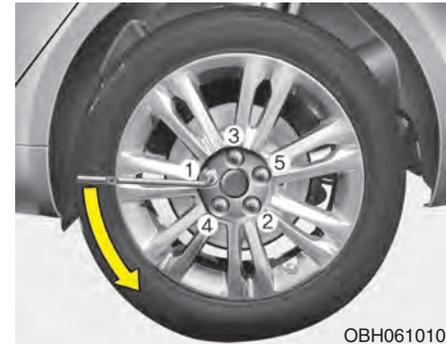
7. Loosen the wheel lug nuts counterclockwise one turn each in sequence of number, but do not remove any nut until the tire has been raised off the ground.
