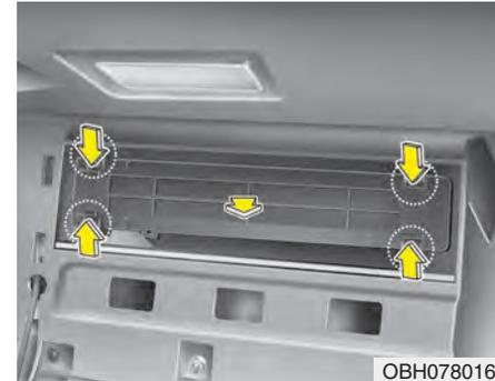
2. Remove the climate control air filter case pulling out both sides of the cover.
