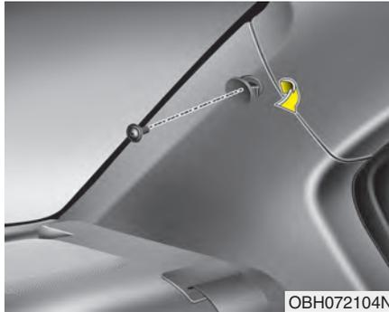
3. Remove the cap, then loosen the mounting screw.
