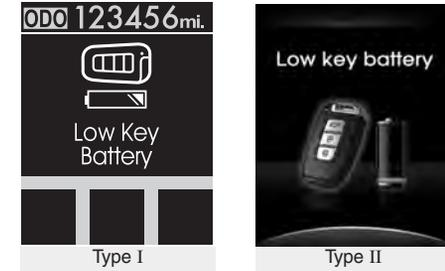
When the smart key in the vehicle discharges, the warning illuminates on the LCD screen for 10 seconds.
