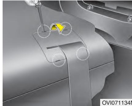
5. Push the hook, remove the rear seat belt cover.
