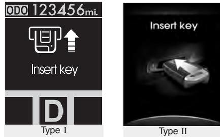
If you push the engine start/stop button while the "Key is not detected" illuminates on the LCD screen, the warning illuminates for 10 seconds.
