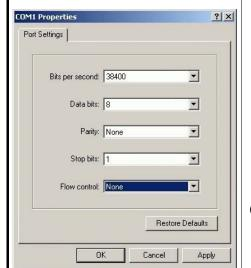
3. Set the COM port parameters according to the settings listed down below:
