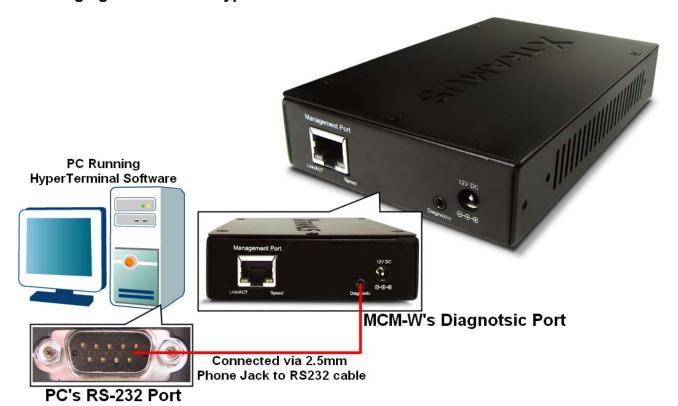
MCM-W allows users to make system configurations and view test statistics/system information with **HyperTerminal**. To access MCM-W via **HyperTerminal**, you have to connect MCM-W's **Diagnostic Port** with **PC's RS-232 Port** via a 2.5mm Phone Jack to RS-232 cable as shown in the figure above.
