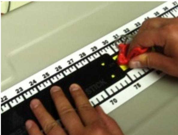
The calibration is complete. Verify the calibration with a measurement of a single cal-stick or some other device of known length. Go into LENGTH-MEASURE mode and place a single cal-stick on the board, allowing the stick to rest on top of the small radius at the nose-stop wall and take a measurement. You should see "375"mm for your measurement. If not, verify you did all of the steps correctly (including verification) and repeat the calibration if necessary.
