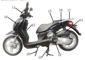
10 Headlight 14 Air filter 18 Kick-start pedal 11 Front turning light 15 Seat 19 Main stand 12 Helmet hook 16 Seat lock 20 Side stand
