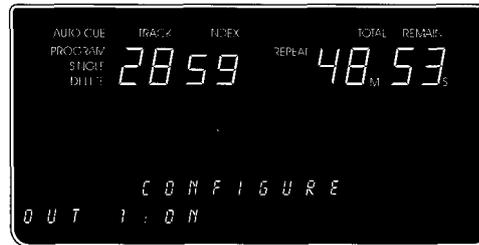
2. The factory setting is ON, so press the VOLUME UP or VOLUME DOWN keys to select between ON and OFF. When OFF has been selected, the display looks like this:
