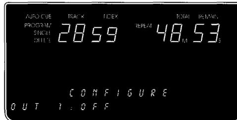
3. The setting is not changed (or saved) until the MUTE key is pressed. NOTE: If you do *not* press any key for ten seconds, the display will revert to the status screen.
