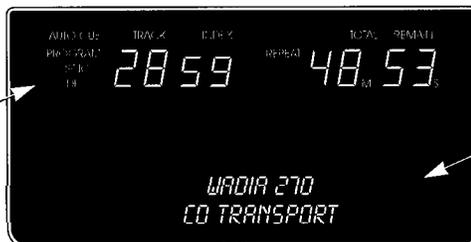
The bottom section is an alphanumeric display that shows the status of some of the Wadia 270 special functions.
