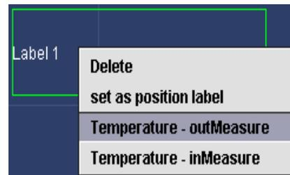
You can write static text (e.g. 1st Floor), or text changing with a Data Point value, e.g. a measurement. A right click gives you a pop-up for the selection of the source Data Point, e.g. temperature measurement.
