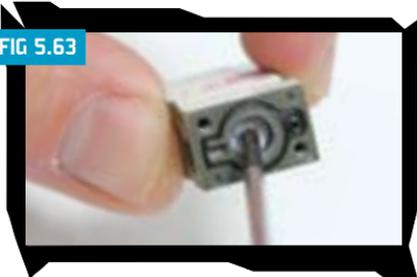
Thoroughly clean and inspect the spool and its O-rings for any debris or dirt (SEE FIGURE 5.64). Lubricate the o-rings using Dow 33 or similar lubricant and re-insert the spool into the solenoid body, with the concave end towards end A of the solenoid body.
