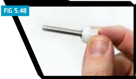
Remembering to include the valve spring, begin to insert the rammer assembly into the Etek2 body. By applying slight pressure to the back of the rammer assembly hold the rammer in place against the exhaust valve spring tension, so that the valve plug can be replaced (SEE FIGURE 5.49).
