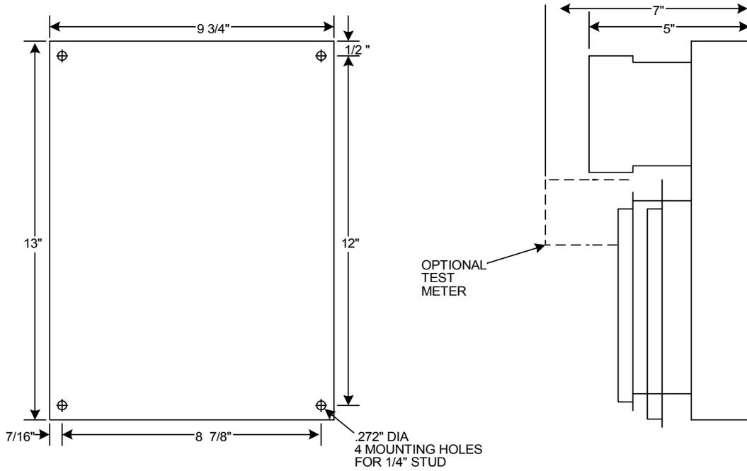
Figure 14: Chassis Mount Control
