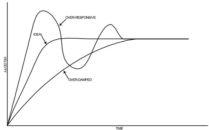
Figure 11: Stability Effects on the Velocity Profile
