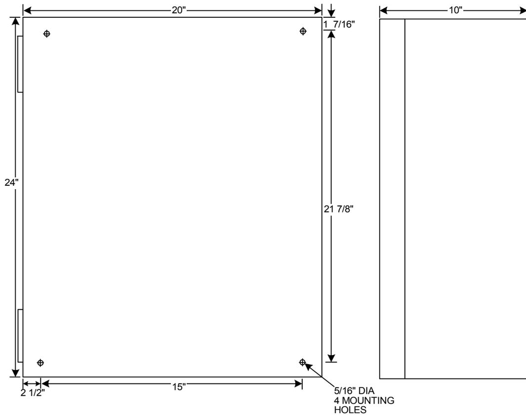
Figure 15: Enclosed Control
