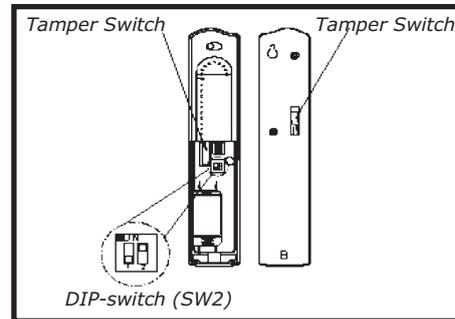
2. DIP switches 1-2 are used to enable/disable the internal or external wired magnetic contact. (FIGURE 3)
