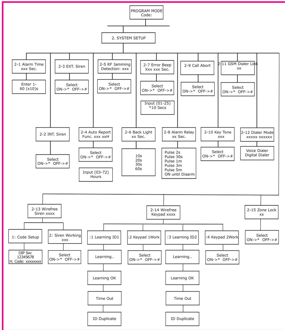
Scroll through the top level programming menu until '2 SYSTEM SETUP' is displayed and press .
