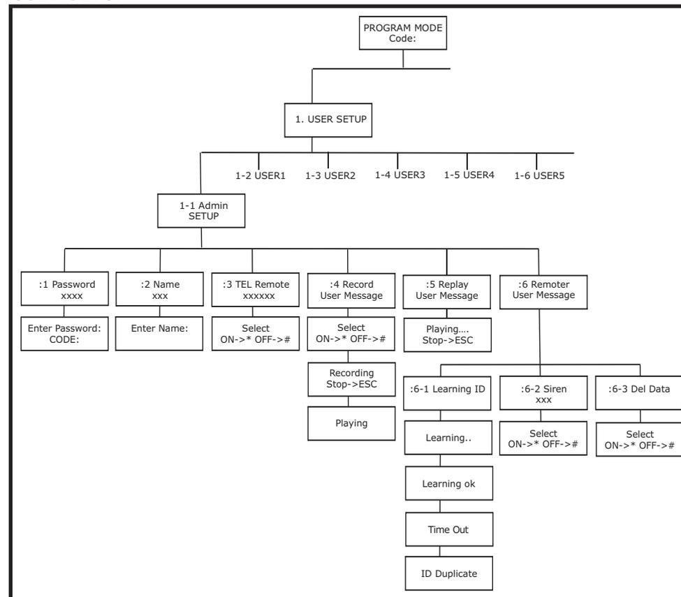
Scroll through the top level programming menu until **'1. USER SETUP'** is displayed and press
