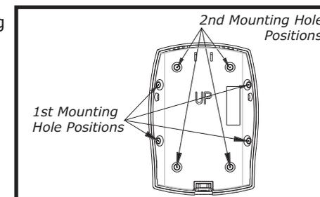
**Note:** Using 1st mounting hole to fulfill corner mounting installation, while 2nd mounting hole for flat wall installation.
