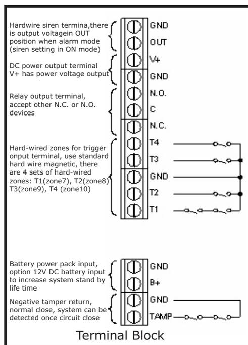
Hardwired zone and tamper switches should be Volt free and Normally Closed, with the contacts opening in order to initiate an alarm.
