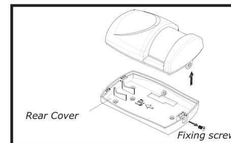
2. Carefully drill out the required mounting holes in the rear cover using 3mm drill according to whether the unit is being mounted in a corner or against a flat wall.
