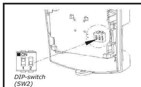
1. DIP1 of SW2 is used to configure the PIR Detector for walk test mode, which allows the operation of the detector to be checked during installation without triggering a Full Alarm.
