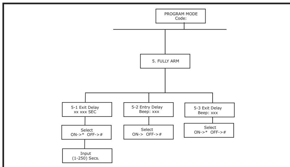
Scroll through the programming menu until '5. FULLY ARM' is displayed and press .
