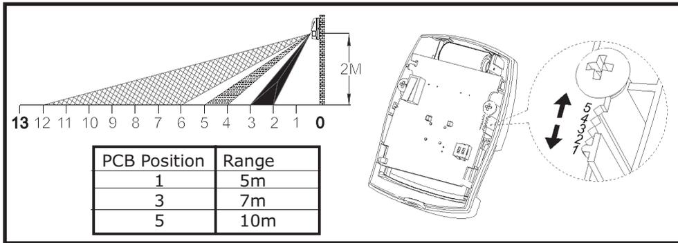
When considering and deciding upon the mounting position for the detector the following points should be considered to ensure trouble free operation:
