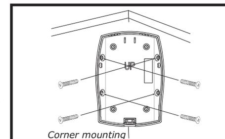
4. Fix the rear cover to the wall using the two 18mm No.4 screws and 25mm wall plugs, (a 5mm hole will be required for the wall plugs). Do not over-tighten the fixing screws as this may distort or damage the cover.
