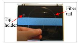
3. Gently push the fiber until the magnetic tip holder is almost fully off the magnet in the box.
