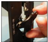
8. Before you close the head, turn the stepper motor counter clockwise to bring the lever further from the head. This leaves more room between the tip and the sample ensuring that the tip does not touch the sample.
