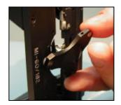
9. Before you close the head, turn the stepper motor counter clockwise to bring the lever further from the head. This leaves more room between the tip and the sample ensuring that the tip does not touch the sample.
