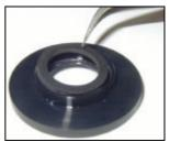
5. Place the washer above the O-ring. Be sure to leave the grooves facing upwards.
