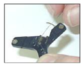
7. Open the NSOM/SPM-100<sup>TM</sup> head and place the tip mount (with tip) onto the three magnets under the head.
