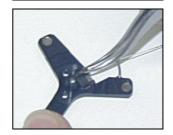
7. Once you have placed the tip onto the mount, gently tuck the tail of the tip under the clip.
