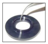
4. Place the rubber O-ring over the cover plate and ensure that it is firmly in place.
