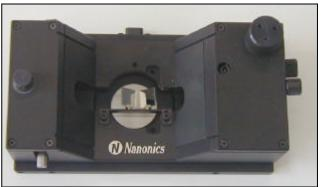
**Note**: The metal bridge, which holds the mirror, can also be used for other applications that require only one mirror. Simply remove one mirror and position the remaining one correctly.
