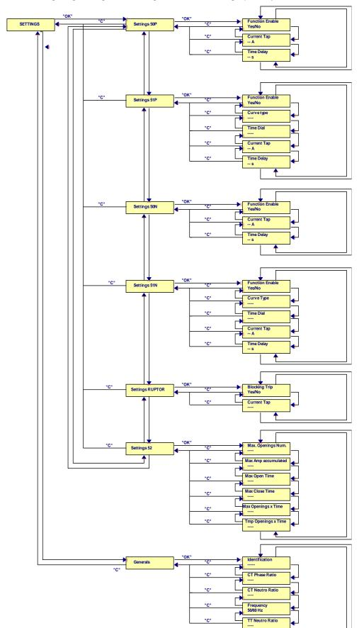
The method for navigating through the settings menu is shown graphically below.
