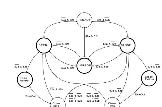
The circuit breaker performance is shown in the following finite state machine:
