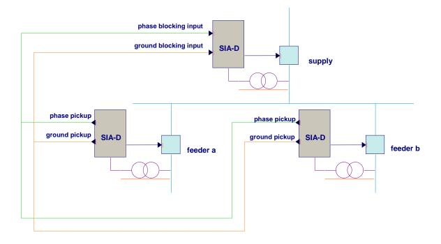
By using relays SIA-D a tripping bus is implemented. Based on the figure, there are 2 relays with the function of feeder and 1 relay with the function of supply.
