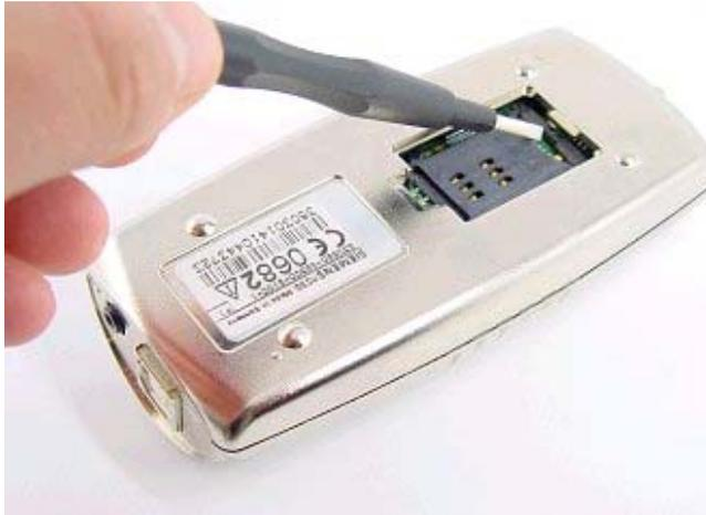
**Fig. 5: Loading the SIM card step 2**
