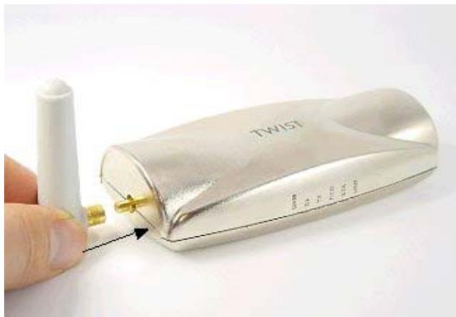
**Fig. 3: Installing the GSM antenna**
