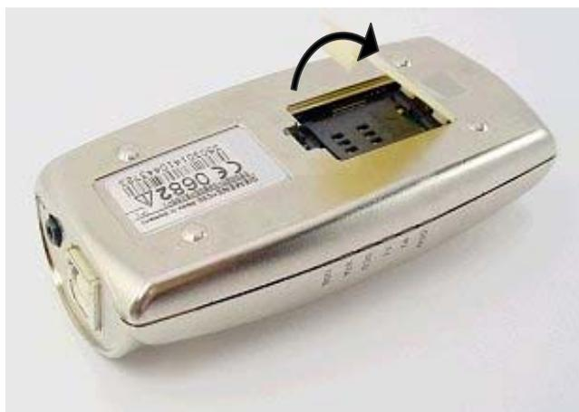
**Fig. 4: Loading the SIM card step 1**
