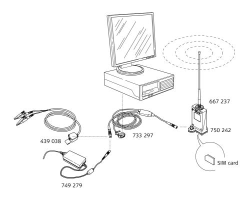
750 242 GFU24, Housing with Siemens MC75 GSM/GPRS Module (Quad-Band GSM 850/900/1800/1900 MHz).
