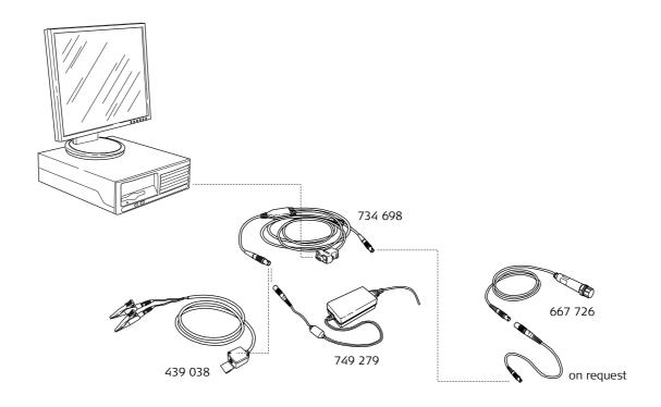
DTM meteo sensor, combined pressure and temperature sensor 2m cable with Lemo1 plug. (other lengths of cable on request).
