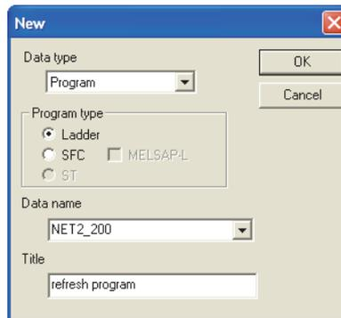
Figure 7.4 Adding new data to a project
