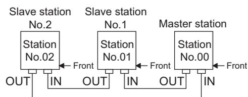
Figure 5.5 Connection method
