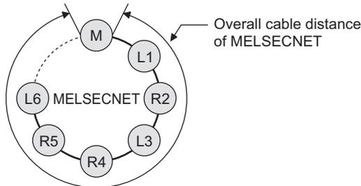
**Figure 3.1 Overall cable distance of MELSECNET**
