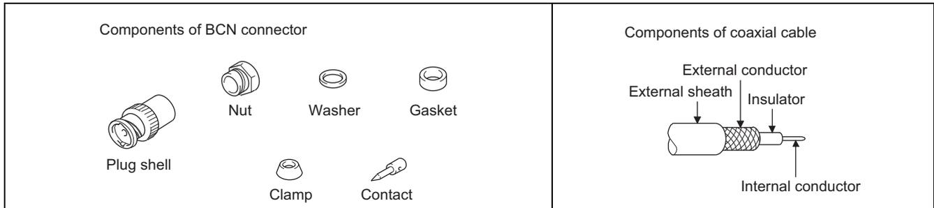
Figure 3.3 Components of BNC connector and coaxial cable
