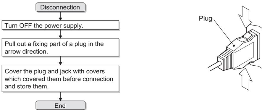
Figure 5.7 Disconnecting an optical fiber cable
