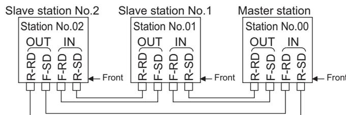
Figure 5.9 Connection method
