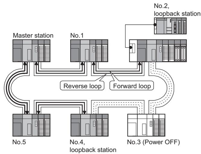
**Figure 4.13** When a local station is powered down
