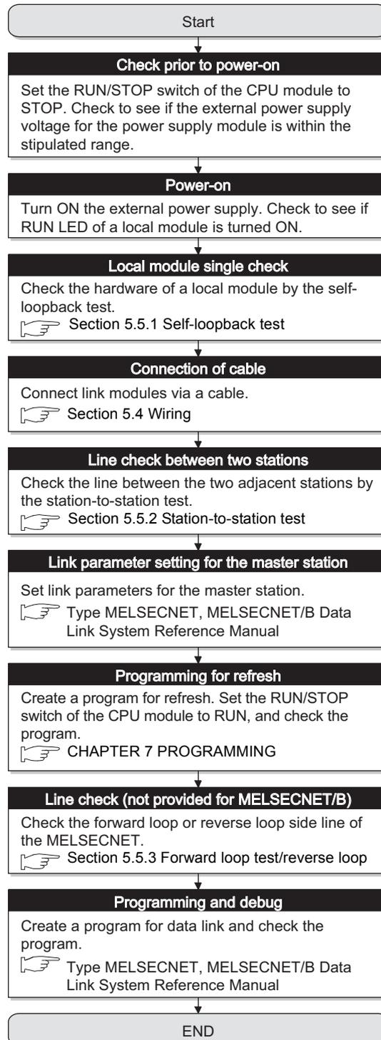
Figure 5.1 Preparatory procedures before operation
