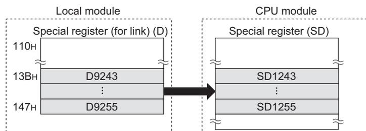
Figure 3.13 Refresh of special register (for link) (D)
