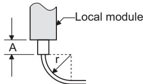
Figure 5.8 Allowable bend radius of coaxial cable
