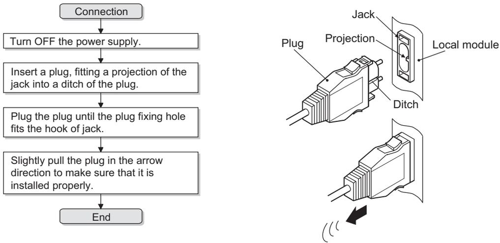
Figure 5.6 Connecting an optical fiber cable
