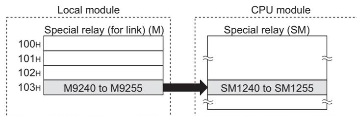
Figure 3.12 Refresh of special relay (for link) (M)
