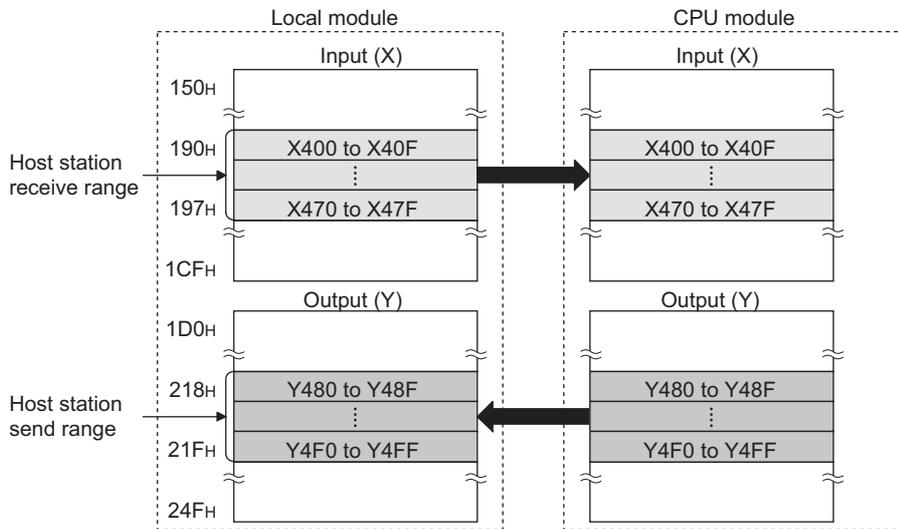
Figure 3.15 Refresh of input (X) and output (Y)
