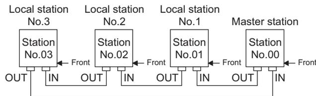
Figure 7.2 Wiring
