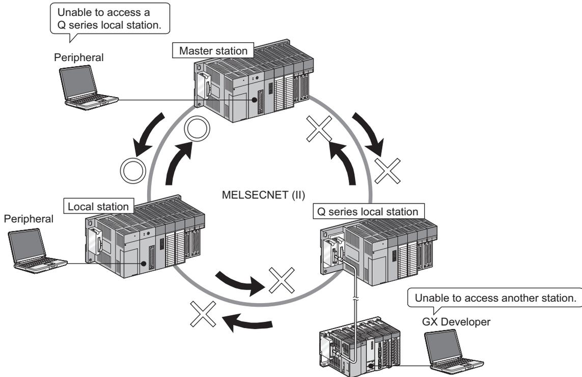
Figure 4.10 Access from a peripheral or intelligent function module to another station
