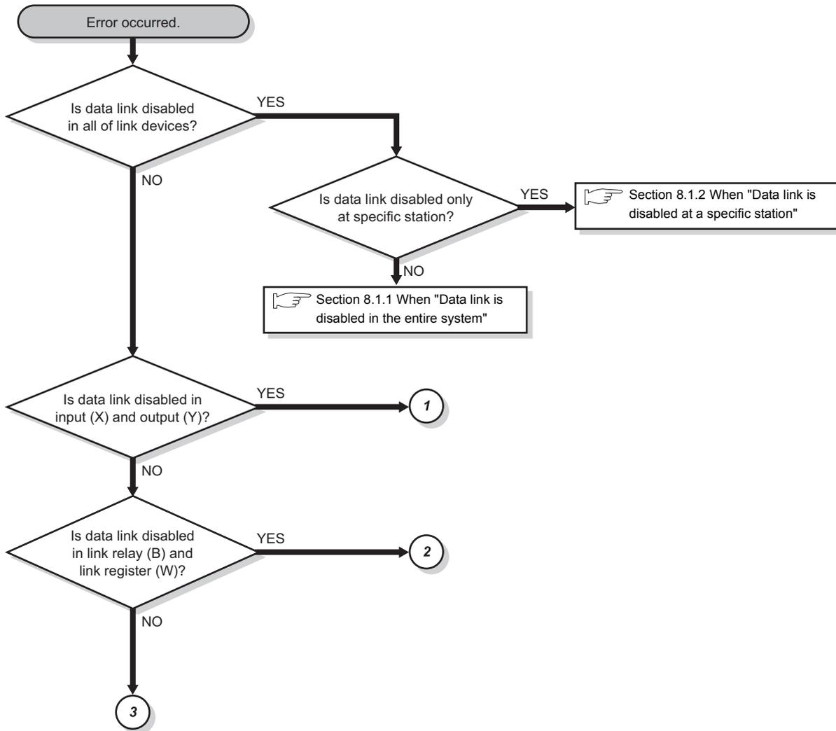
Figure 8.6 When "Error is found in data transmission"
