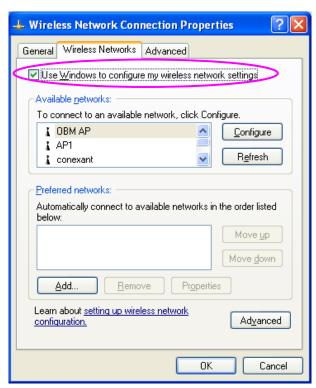
Note: If "Wireless Zero Configuration" is enabled, you can only configure the advance setting or check the link status and statistics from the configuration utility of the adapter.
