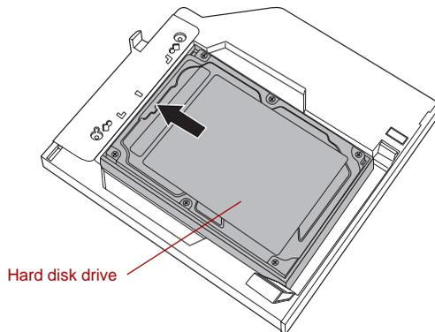
*Figure 3-23 Inserting the hard disk drive*
