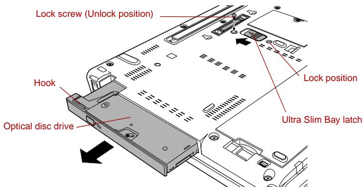
Figure 4-19 Removing the optical disc drive
