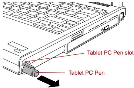
Figure 4-3 Removing the Tablet PC Pen
