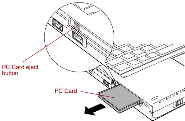
*Figure 3-2 Removing the PC Card*
