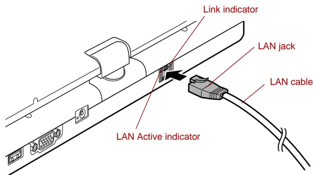
*Figure 4-30 Connecting the LAN cable*
