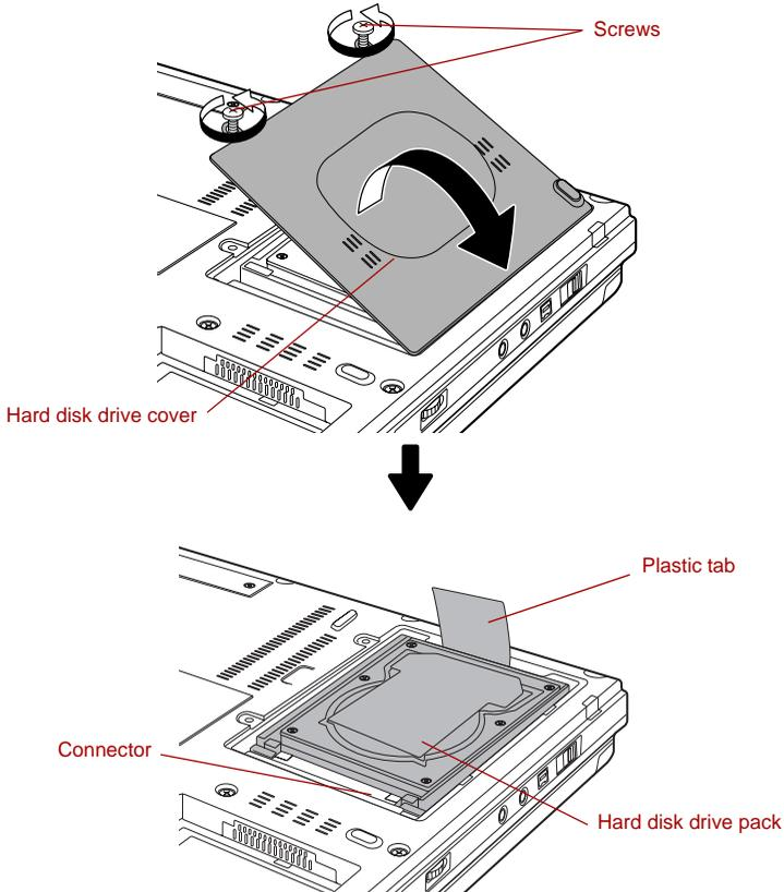
Figure 3-19 Removing the hard disk drive cover
