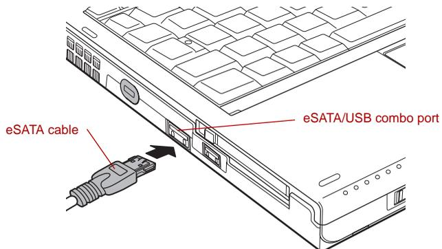
*Figure 3-28 Connecting an eSATA cable to the eSATA/USB combo port*
