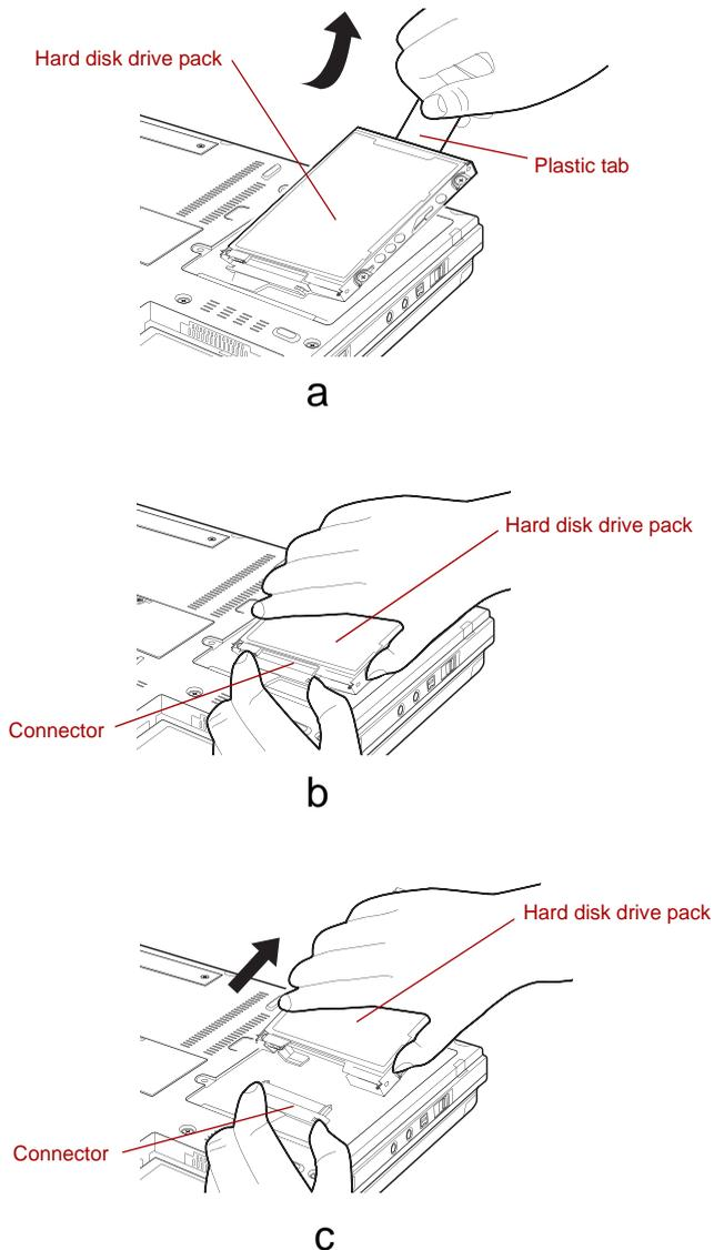
Figure 3-20 Removing the hard disk drive pack
