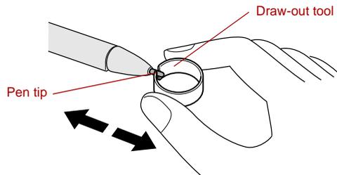
Figure 4-5 Replacing the pen tip
