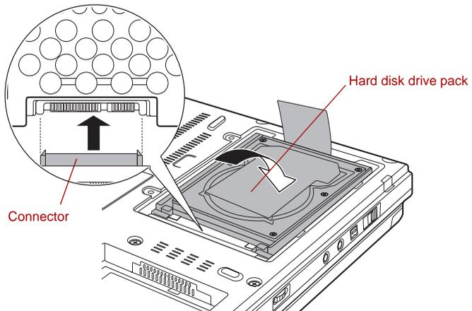
Figure 3-21 Installing the hard disk drive pack
