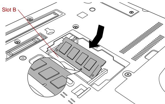
*Figure 3-16 Seating the memory module*
