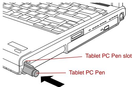
Figure 4-4 Inserting the Tablet PC Pen
