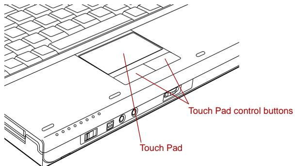
*Figure 4-1 Touch Pad and Touch Pad control buttons*
