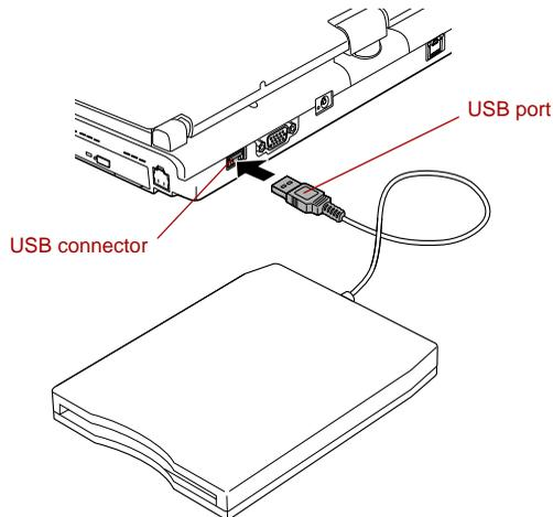
Figure 3-27 Connecting the USB floppy diskette drive
