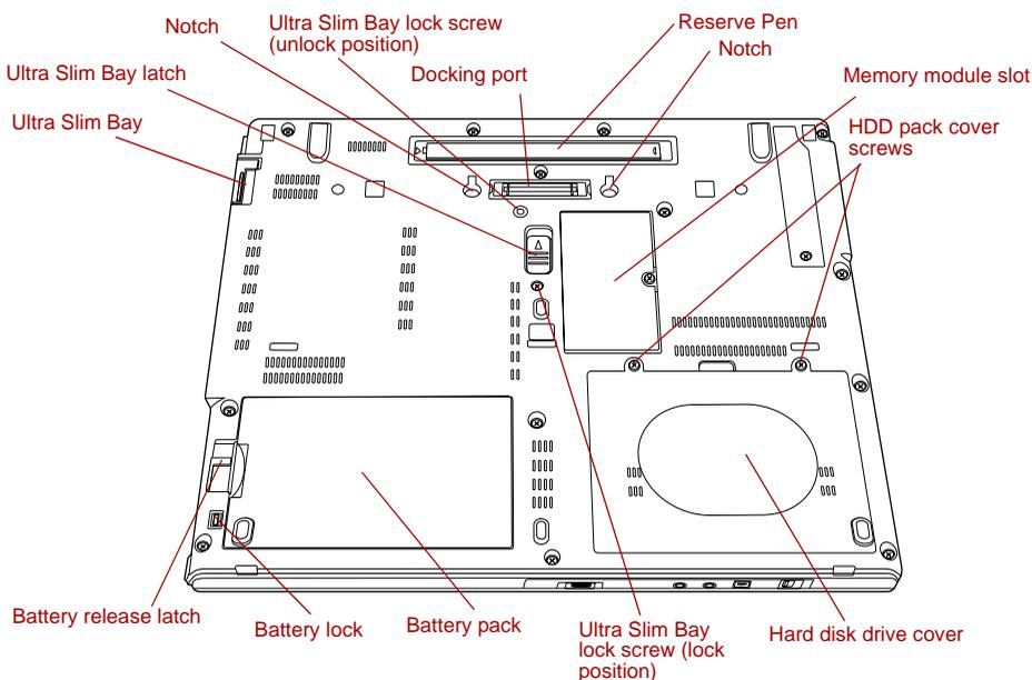
Figure 2-5 The underside of the computer
