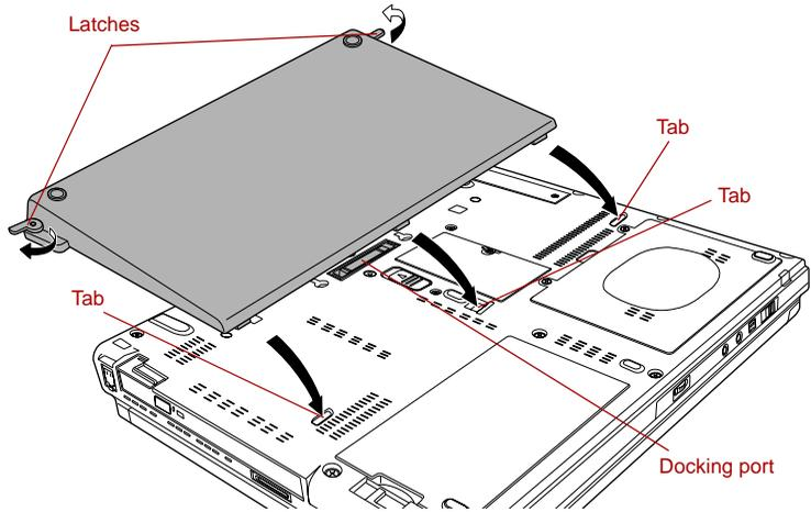
*Figure 6-4 Seating the Slice Expansion Battery*
