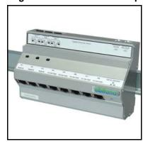
8 full GbE ports with nonblocking wire-speed performance. The ports automatically recognise all attached network equipment and choose the highest possible bit rate (10, 100 or 1000Mbps) and transmission mode for each equipment. The auto MDI/MDIX function eliminates the need (and risk of errors) for crossover patch cords.
