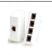
Splitter from one RJ45 jack to 4 RJ45 jacks. Each pair of the RJ45 jack is copied to pair 1 (pins 4&5) of the 4 RJ45 jacks. Can be used to connect four phones over a single cable link. Do not use for Ethernet, video or TV applications.
