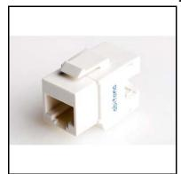
Unshielded RJ45 connector to terminate UTP cable. Used for data and telephony applications. Standard keystone latch makes it compatible with a wide variety of faceplate brands and finishes (lists available on demand) or a keystone patch panel like ABI-HE3002S24.
