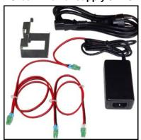
5VDC-4A power supply with a daisy-chain 4-plug output power cord. The cord length between succesive plugs is approximately 40cm, in order be able to reach modules situated far away from each other in a cabinet.
