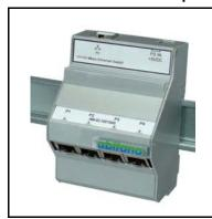
The 5 port 10/100Mbps Switch automatically recognises all attached network equipment and chooses the highest possible bit rate (10 or 100Mbps) and transmission mode for each equipment. The auto MDI/MDIX function eliminates the need (and risk of errors) for crossover patch cords.
