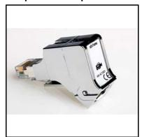
Video adapter to connect an analog camera or camcorder to a universal OmniMedia wall outlet by means of a standard video coax patch cable. Ensures impedance matching (100-75 Ohm). A pair can be used to set up a short RCA-RCA video extension, a single unit can be used to bring a video signal to the ABI-EV1017S00 modulator or the ABI-EV1018S00 active AV splitter.
