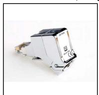
Adapter to connect a TV set or a digital settopbox to a universal OmniMedia wall outlet using a standard RF coax lead. Ensures proper impedance matching (100-75 Ohm). In combination with coax gender changer ABI-CX1005S00 this adapter can be used to connect an FM or DAB radio or tuner. Adapter ABI-AC1030S00 allows the simultaneous connection of a TV and a Radio from a single RJ45 socket.
