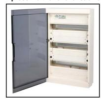
Comm Center cabinet in polymer for wall surface mounting or partially recessed mounting. Fitted with DIN-rails, frontpanel and smoked transparent door. Suitable for small to medium size projects. On the -S22, -S33, -S44 models the frontpanels and side cover of the cabinet can be removed while patch cords stay in place, facilitating add-ons and changes with the system up and running.
