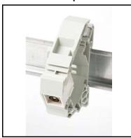
Ensures a quick termination of connectorised coaxial cables in the Comm Center cabinet. Frontside IEC male connector, rear side F coax connector. The keystone latch mechanism maintains the connector in the DIN-rail holder. Adapted for wideband audio/video applications.
