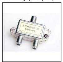
Coaxial wideband 2-way splitter (or combiner). 1 F connector in, 2 F connectors out. 75 Ohm impedance. Used to split antenna, CaTV or modulator signals to separate amplifiers.
