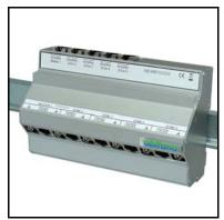
The Multiroom MultisourceModule allows you to create a simple multiroom audio system by interconnecting the music sources from different rooms with audio amplifiers in the central cabinet. Connections to the music sources and to the amplifiers are through RJ45 ports, greatly simplifying the installation work.
