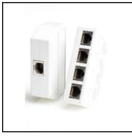
Splitter from one RJ45 jack to 4 RJ45 jacks. All pins of the RJ45 jack are copied 1 to 1 to the pins of the four RJ45 jacks. Can be used to put several high impedance devices in parallel. Do not use for Ethernet, video or TV applications.
