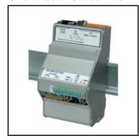
The 2x20W RMS stereo Class D audio power amplifier provides Class AB amplifier performance with Class D efficiency. This device works from a single 14VDC supply, has click-and-pop suppression as well as short-circuit and thermal protection.
