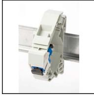
Fiberoptics multimode simplex SC feedthrough connector. The keystone latch mechanism maintains the SC connector coupler in the DIN-rail holder. Occupies 1 standard width on the DIN-rail. The device allows quick termination of Fiber access, backbone or FTTH links in a user premise, industrial site, automation equipment, etc.
