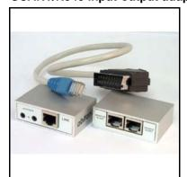
Bi-directional adapter to connect either an audio/composite video source (DVD player, satellite decoder, video recorder,...) or display (TV set, monitor, beamer,...) equipped with a SCART connector to a universal OmniMedia wall outlet through standard RJ45-RJ45 patch leads. Bi-directional IR-Bus interface for remote control transmitter or receiver wands. A unit can be used to bring AV signals to the ABI-EV1017S00 modulator.
