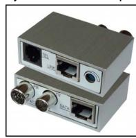
Triple-play adapter to connect a TV set, a digital settopbox and an FM tuner to a universal OmniMedia RJ45 wall outlet using a standard RF coax and RJ45 patchleads.
