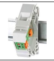
DIN-rail mounted speaker terminal to terminate standard speaker cable up to 2x2mm² in a DIN-rail cabinet. Perfectly suited to prewire a home for stereo or surround multiroom audio. The spring loaded contacts accept solid or stranded wires and retain good contact even in case of wire sagging
