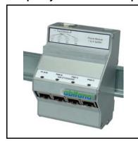
This module allows the transmission of 4 individual analog or digital 2-wire phone signals over a 4-pair twisted pair cable. The 4 pairs present on an RJ45 connector (top) are split and each one sent to an RJ45 on the module's front. The module can be used in both directions, to either split or combine signals onto a single cable.
