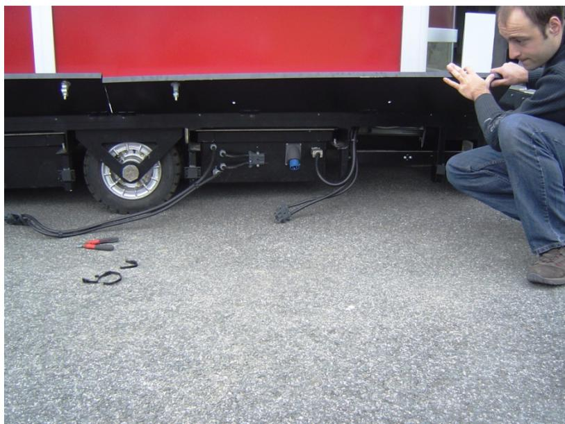
**Figure 2 - The training course in Robosoft premises – how to pull out battery rack.**
