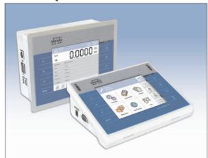
PUE 7 weighing indicators are intended for building industrial scales. It can be enclosed in a plastic or stainless steel housing for rack installations. It is equipped with a 5.7" colour graphic display with touch panel and membrane keypad. It also has installed two proximity detectors with programmable functionality.
