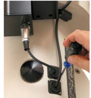
6. Connect Cable and Attach Port Plate
