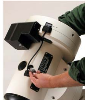
3. Feed Cable through Cable Port
