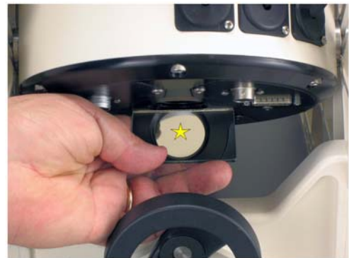
Rough Polar Alignment with a Small Flat Mirror
