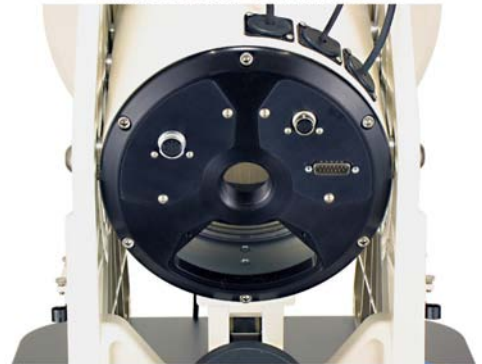
Auxilliary Cable Port Cover Plate and Rear Sight-Hole Cover Removed
