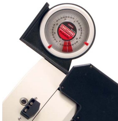
Sighting Polaris through Polar Alignment Sight Hole
