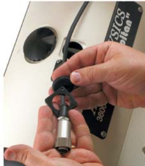
4. Add Cable Port Plate - Flat side out
