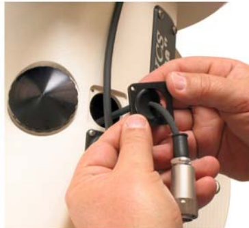
5. Carefully work Grommet onto Cable Port Plate
