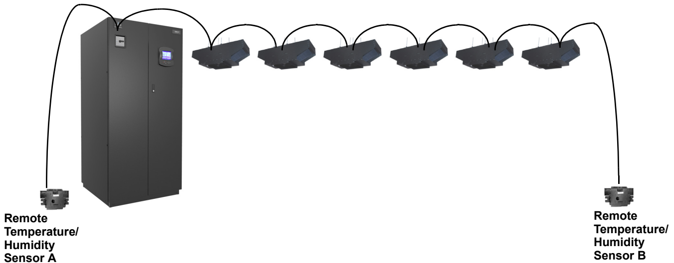
Figure 44 Liebert XD system with CANbus
