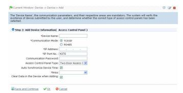
**IP** Address: Please enter the IP Address of the access control panel;
