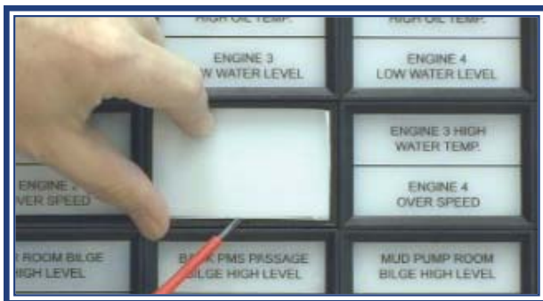
4- Insert the screwdriver inside the slot and lever the lens forward
