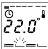
During the timer programs, P2, P3, and P4, the flashing
