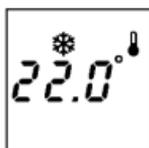
The thermostat is now in frost protected mode. Actual temperature is shown.
