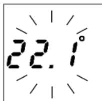
Use the arrow buttons  $\blacktriangle$   $\blacktriangledown$  to either increase or decrease the temperature. The temperature is changed in increments of  $0.1^{\circ}\text{C}$ .
