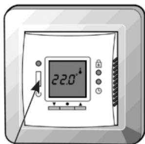
This is a safety switch, meaning all electrical supply to the thermostat is disconnected when turned off.
