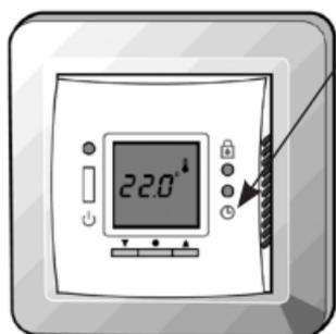
You enter the settings by pressing the ⌚ pinhole with a small screw driver, pencil, or needle, the display now changes from temperature to time display.
