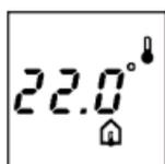
If installed as a combination thermostat, by pressing ▲ and ▼ at the same time for 2 seconds, the temperature in the floor sensor is displayed for 2 minutes. The floor sensor icon 🏠 is displayed.
