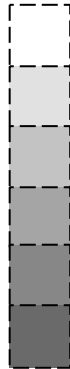
Figure B.2.6.5.1. A 6-step greyscale to be used for the measurement of colour greyscale linearity. Each square is 40 mm × 40 mm in size.
