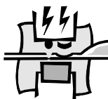
1-2 CUT-OFF SEAL 1 x 3,5 mm seal 1 x 1,1 mm cut individual time
