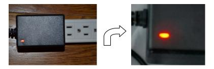
Once fully charged the LED will turn Green. Unplug the charger and disconnect the battery.
