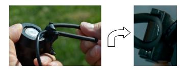
Place the light head on the handlebars and stretch the O-ring around the bottom of the handle bar. Clip it onto the hook at the rear of the light head. Various O-ring sizes are provided; Use the one which provides the best fit depending on the size of your handle bars.
