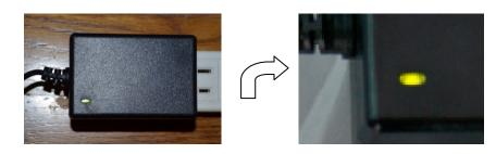
• Plug the charger into the power outlet – the charger LED will turn Red indicating that the battery is charging. A full charge from empty will take approximately 4 hours.
