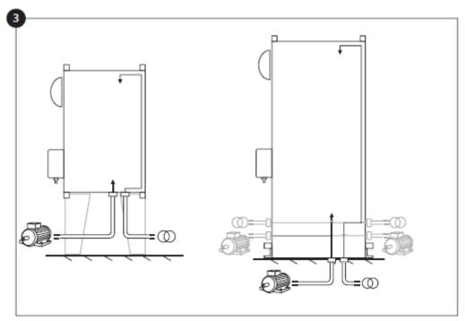
Make sure to drill holes for the motor and power connections and run the cables inside the panel, all in accordance with the specifications in order to minimize interference with other equipments.
