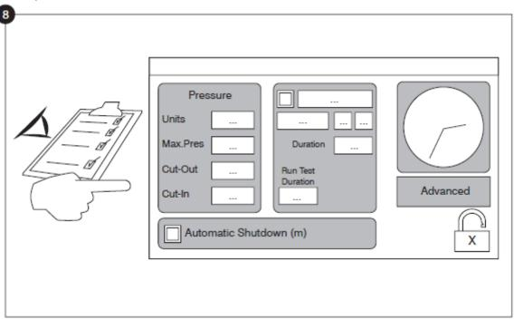
Select the controller pressure units, cut-in and cut-out. Verify that all other parameters on the setup page are correct.
