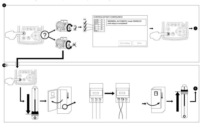
Verify the motor rotation to insure that the pump is turning in the right direction. The START and STOP push buttons can be used to toggle the motor ON/OFF.
