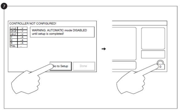
The "First Setup" page replaces the Homepage until the "First Setup" is done. Proceed to the setup page and press the lock to enter your authorization code.
