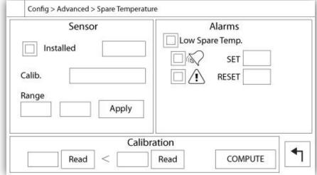
In the ViZiTouch, all sensors refer to analog input connectors on the I/O board. They all have similar settings and configuration.
