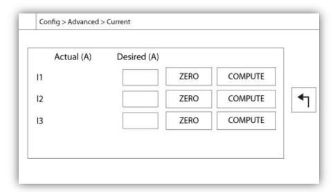
To calibrate a particular current sensing element, enter the current value as read from a calibrated ammeter and then press COMPUTE. For best results, press the ZERO button when no current is flowing through the sensing element before calibrating.
