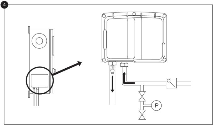
Verify and/or install the proper water connections for the water input and the drain. They must be securely installed and tightened. Refer to the silkscreen markings on the plastic cover.
