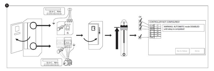
Connect the input power and the motor on their respective terminals. Secure with the appropriate torque as indicated on the torque label and verify all connections. Secure the door in closed position then put the circuit breaker disconnecting means in ON position. Verify the readings on the controller main screen.
