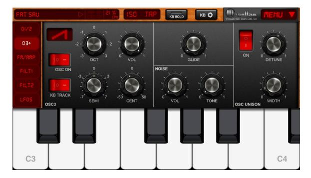
The KB TRACK toggle is used to couple oscillator 3 to the keyboard/controller input. In the OFF position, oscillator 3 is decoupled and operates as an audible LFO. In the ON position, oscillator 3 works like oscillators 1 and 2.
