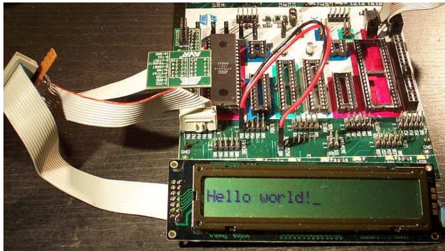
Figure 5: Wiring of the STK500
