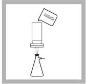
**4.** Rinse the filter by pouring approximately 50 mL of deionized water through the filter. Discard the rinse water.
