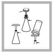
**3.** Assemble the filtering apparatus (0.45 micron membrane filter, filter holder, filter flask and aspirator).
