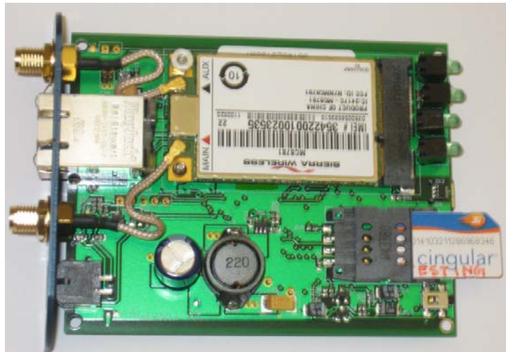
Figure 3-3: Insert SIM in to the modem
