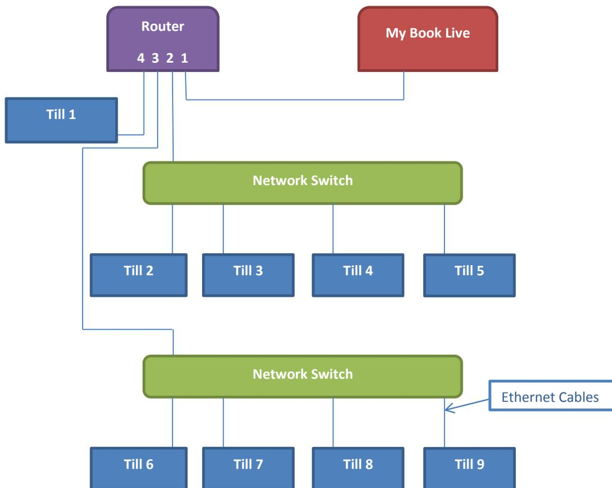
Each till consists of a laptop, USB barcode scanner and USB printer.
