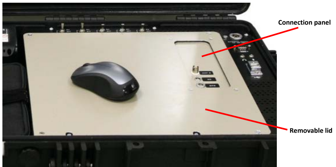
Figure 4 MEC protection lid with configurable connection panel.
