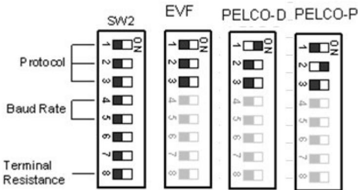
**Notice:** Please make sure the power is off before setting, and restart the EPTZ860 to enable a new value after changing.
