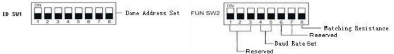
**Note:** You will see the label of Protocol & Baud Rate as well as RS-485 ID address show on the speed dome. White part represents the switch key. For example: for EVF protocol, white keys are all switched downward; for ID Address 0, white keys are all switched downward.
