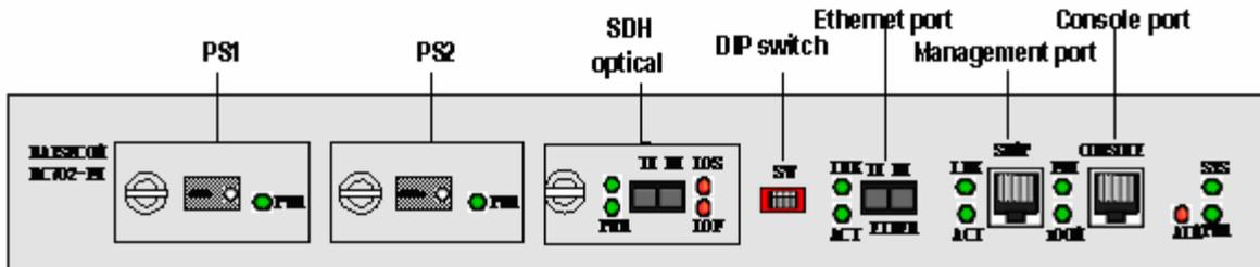
Figure 4-1 RC702-FX with SDH optical port
