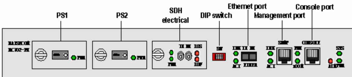
Figure 4-2 RC702-FX with SDH electrical port
