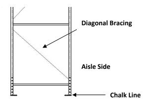
Upright frames should be positioned so that the lowest diagonal bracing is pointed downward toward aisle side
