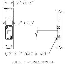
BOLTED CONNECTION OF ROW SPACER (RSC) TO CHANNEL UPRIGHT (BCF)
