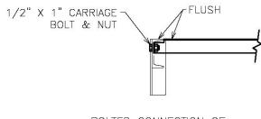
BOLTED CONNECTION OF PALLET SUPPORT (PSB) TO CHANNEL BEAM (CB7)
