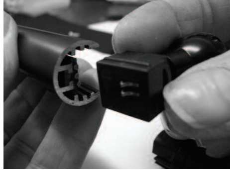
Incorrect - pins facing the wrong way
