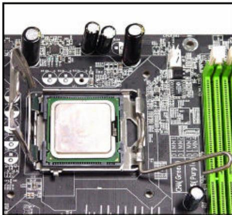
8. Cover the load plate onto the package.
